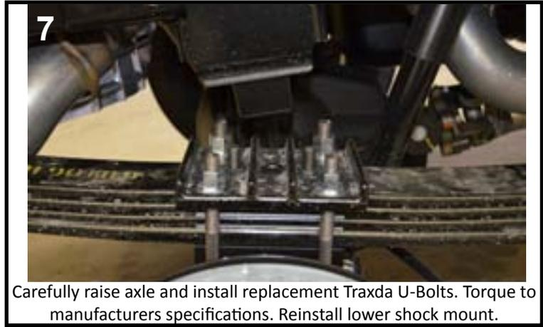
Carefully raise axle and install replacement Traxda U-Bolts. Torque to manufacturers specifications. Reinstall lower shock mount.
