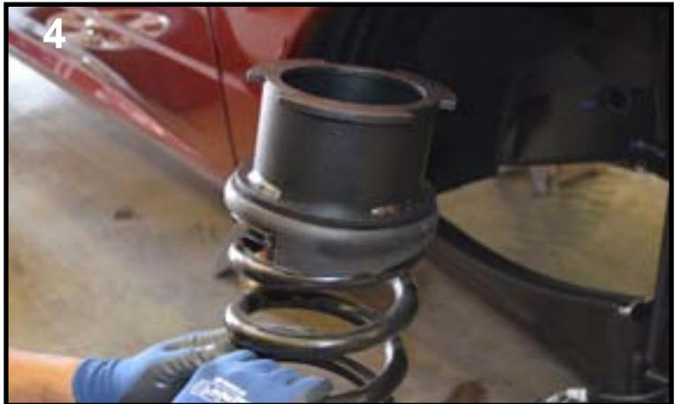
Re-install the isolator onto the spring, and mount the Traxda Coil Spacer above it. Repeat steps 3 and 4 for other side of vehicle.
