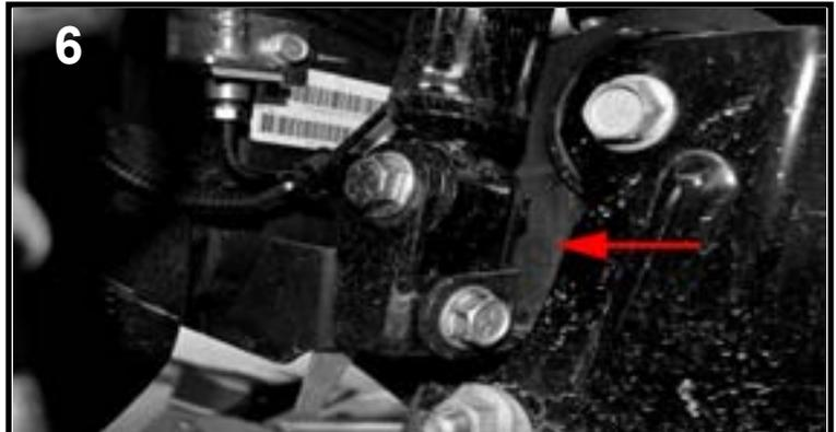
Install Traxda Shock Extensions onto bottom of shocks with provided hardware. Using factory hardware attach extensions onto axle.
