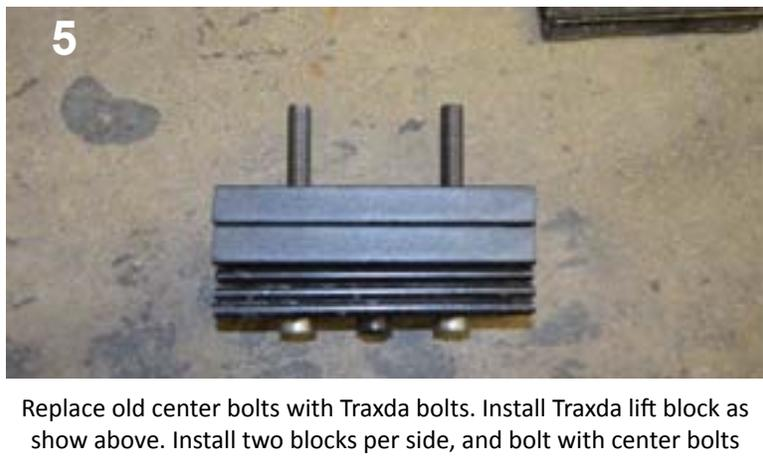
Replace old center bolts with Traxda bolts. Install Traxda lift block as show above. Install two blocks per side, and bolt with center bolts
