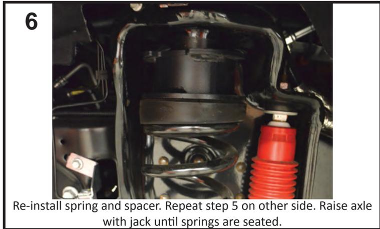
6 Re-install spring and spacer. Repeat step 5 on other side. Raise axle with jack until springs are seated.
