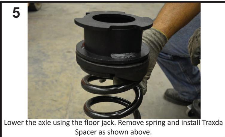
5 Lower the axle using the floor jack. Remove spring and install Traxda Spacer as shown above.
