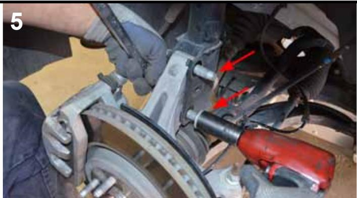
Remove the lower strut mounting bolts from the spindle. you may need to carefully tap the bolts with a hammer to fully remove them.
