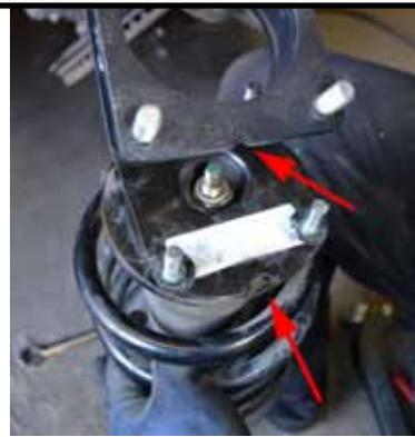
Install spacer on strut using factory nuts. Align notched edge with curved edge of strut mount. Reinstall in vehicle with curved edge facing away from engine.
