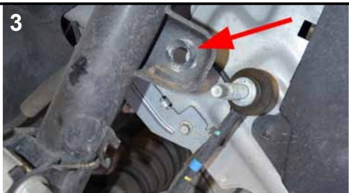
Disconnect sway bar end link from strut.
