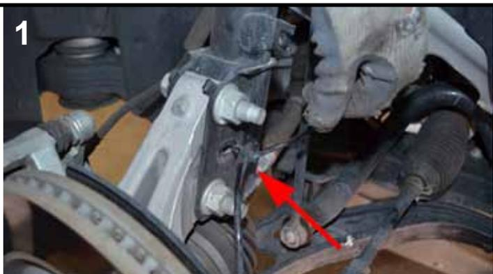
Raise vehicle on jack stands and remove wheels. Disconnect the ABS and brake hose.
