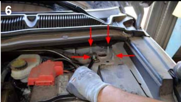
Remove nuts from upper strut mount. Support weight of strut before removing final nut. Remove strut from vehicle.
