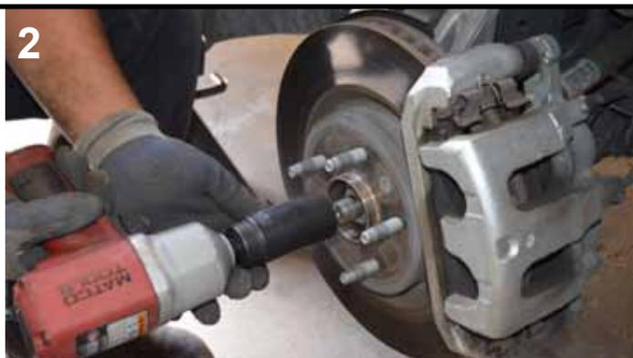
Loosen & remove the axle nut, and push the axle through the spindle.
