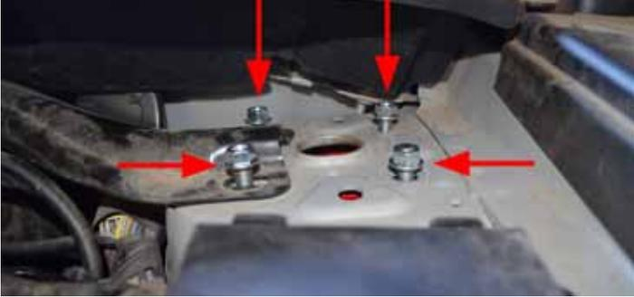
Reinstall upper strut mounting nuts. Do not tighten fully.
