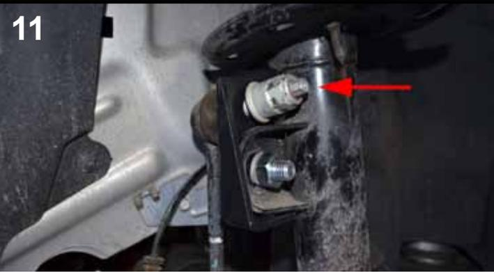
Install Traxda sway bar extension bracket with provided hardware. Tighten the sway bar end link to the Traxda bracket.
