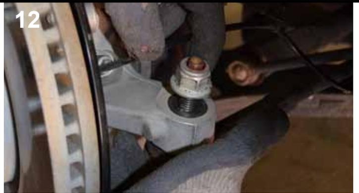
Re-tighten the axle nut, reinstall the tie rod (above) and the ABS/brake lines.
